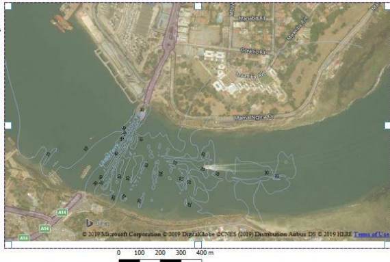
A satellite map of the Likoni Channel generated using acoustic data
