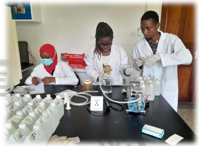
KMFR I team Josephine Kerubo and Douglas Mandela perform filtration of water samples to analyze Total Suspended Solids (TSS) and chlorophyll. Chlorophyll is a key component for productivity as a primary provider of energy in the food chain. TSS is being analyzed because in high concentration it reduces water visibility and clogging in the fish gills hence leading to death and also prevents the penetration of sunlight in the water
