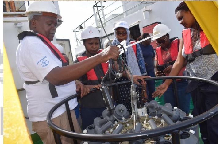
Top, KMFRI researchers and Kenya Coast Guard Services team. Below, cruise leader Dr Mbaru (2nd left) with researchers and technologists prepare CTD rosette for deployment
