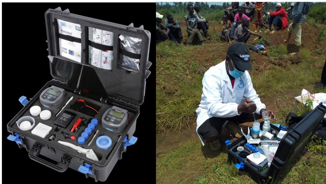
Plate 1. Portable Field Incubator for field water microbiology test.
