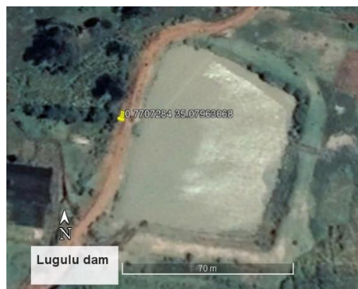
Plate 25. Lugulu dam is located in Likuyani sub-county at an altitude of 1776 m around the GPS points, 0.7703, 35.0802. The appearance of the dam is Milky from clay/rock sediments. Inflow of clear water from a natural spring, with cement channelized at the inlet. Outflow is through a spill way into the continuing stream.
