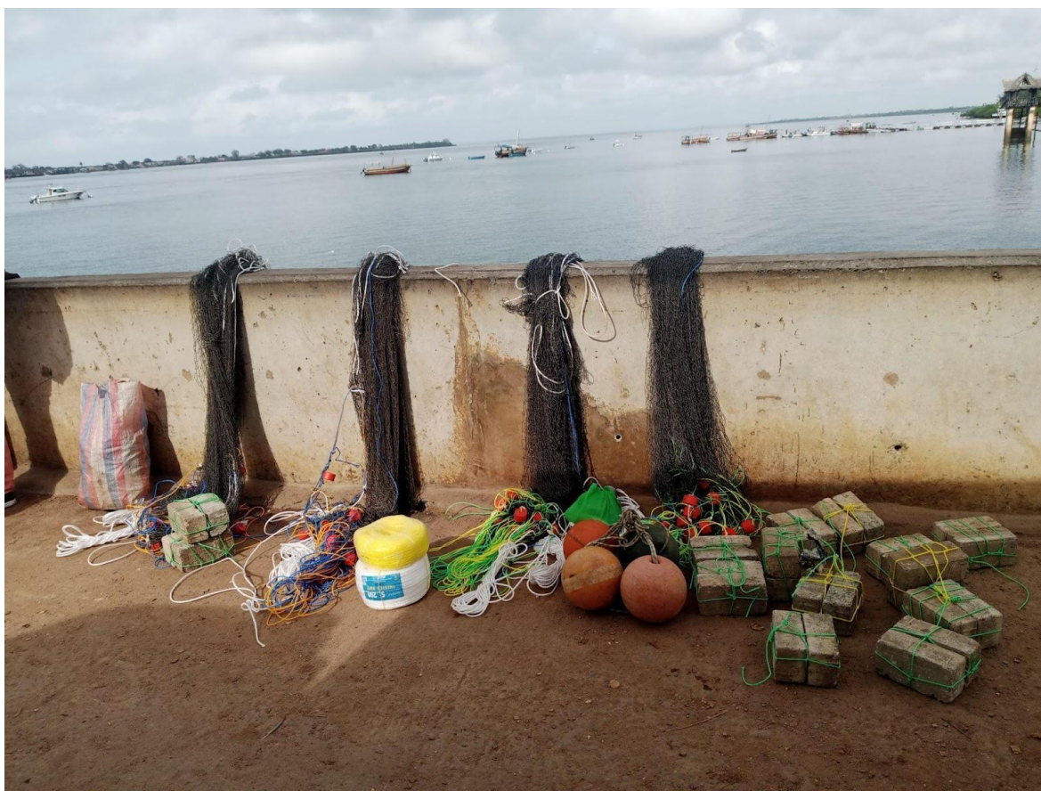
Picture 4: 30m by 2m size modified nets for the degradation testing experiment
